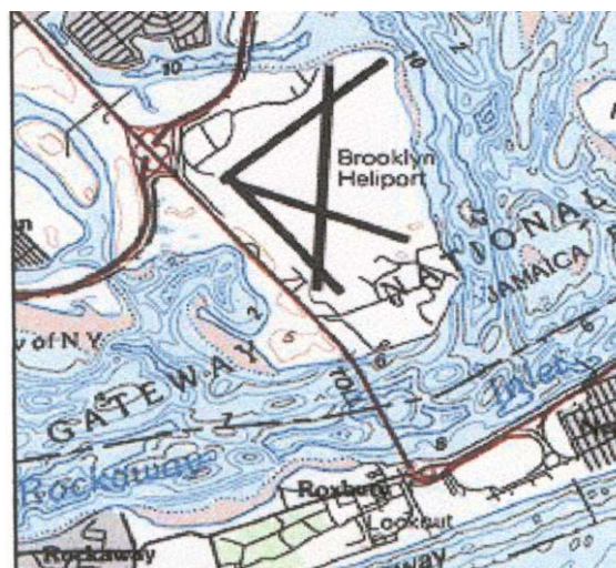
Figure 11. Floyd Bennett Field was built on organic soils (Ipswich, Pawcatuck, Matunuck) and eolian sediments (Hooksan) using dredge material from Jamaica Bay.
