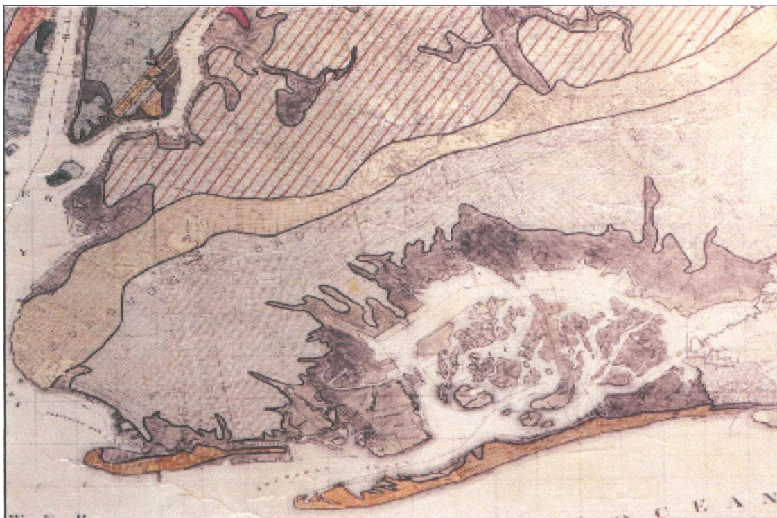
Figure 5. The terminal moraine (yellow) marks the maximum extent of the ice sheet. Outwash plains (white) were formed by meltwater stream deposits. Organic deposits (black) formed 4,000 years ago in a lagoon protected by barrier beaches (orange) (courtesy of NYC-Department of General Services, Subsurface Exploration Section).
