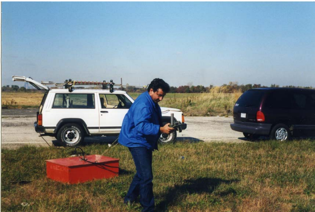
Figure 52. Soil Scientist using Ground Penetrating Radar to map and detect subsurface soil features.
