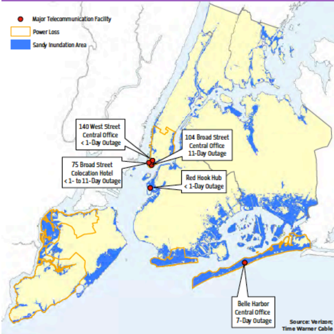
Major telecommunications facility outages during Sandy. Source: p. 165 City of New York (2013).
